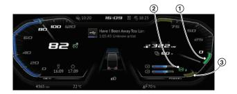
The available power can be limited by certain conditions. Battery State of Charge, temperature, and the motor temperature may trigger the limitation, at which point yellow blocks will be visible in the Digital Instrument Panel. This yellow visual overlay (3) represents the amount of power not available. The green bar (1) shows the amount of energy that is currently being recuperated (braking power). The green telltale (2) shows the activation and, if applicable, level of e-Drive Control.
