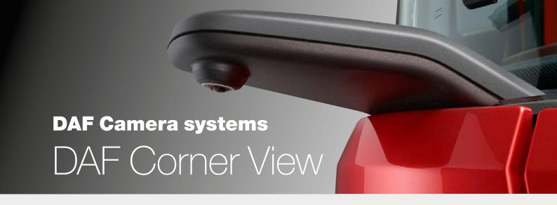
To improve vision and safety around the cab, especially in urban environments, DAF has introduced the DAF Corner View (option 01913). A wide-angle camera, fitted to the corner of the cab on the co-driver side, which replaces the kerb view and front view mirror. In addition to offering superior vision around the cab. the aerodynamically shaped camera is also beneficial for fuel efficiency.
